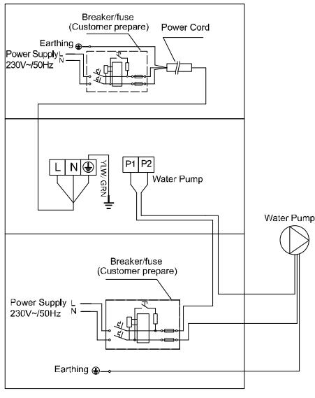
For water pump: Voltage 230V, Capacity >500W
