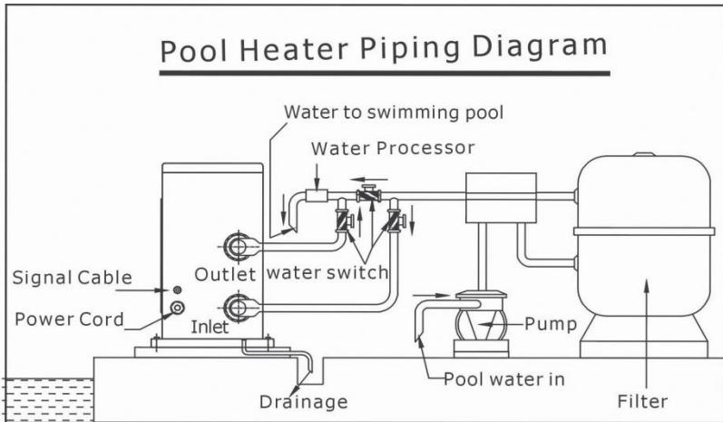
(Notice: The drawing is just for demonstration, and layout of the pipes is only for reference.)
